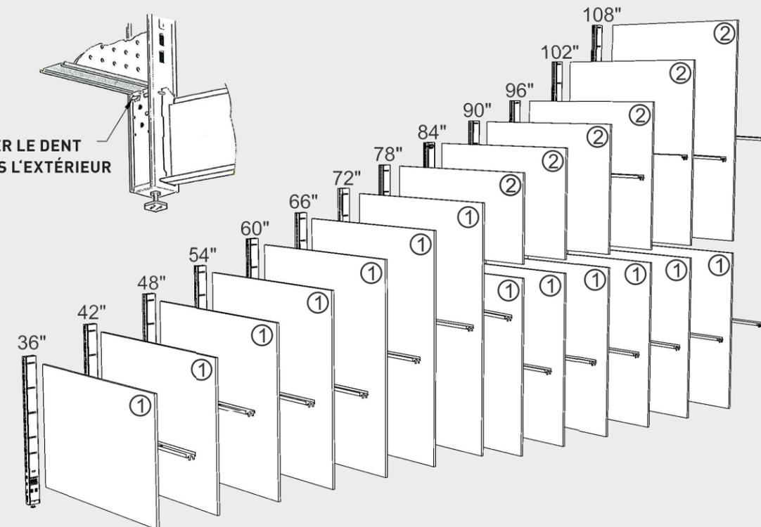
AFIN DE STABILISER LA STRUCTURE, INSÉRER LA PLINTHE OUVERTE (ITEM#9) SUR LE DEVANT DES PIEDS ET INSTALLER LA TABLETTE DE BASE (ITEM#8) EN S'ASSURANT QUE LES DENTS SONT INSÉRÉES DANS LE BAS DU POTEAU.
