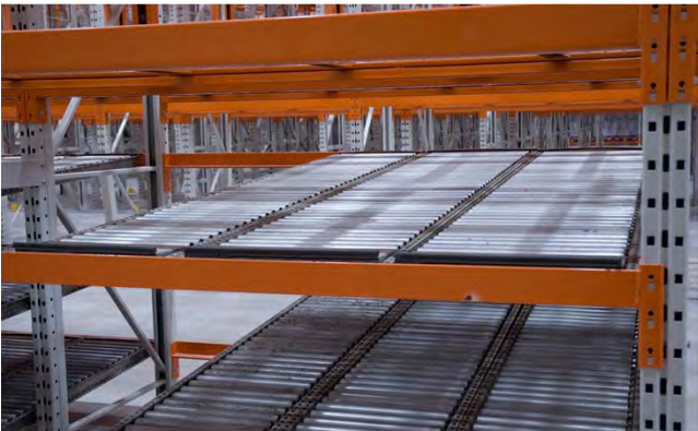
Gravity-flow racking system
