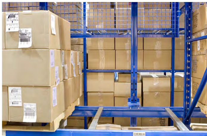
Pallet stopper and protective wire panel
